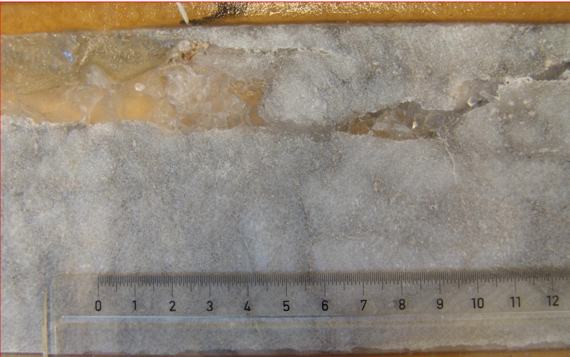
Tubbergen-7, 1490.8m AH ZE2A. Halite filled fracture in Anhydrite.
