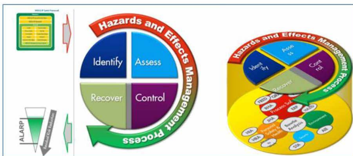
Fig. 3.2: Hazards & Effects Management Process (HEMP)
